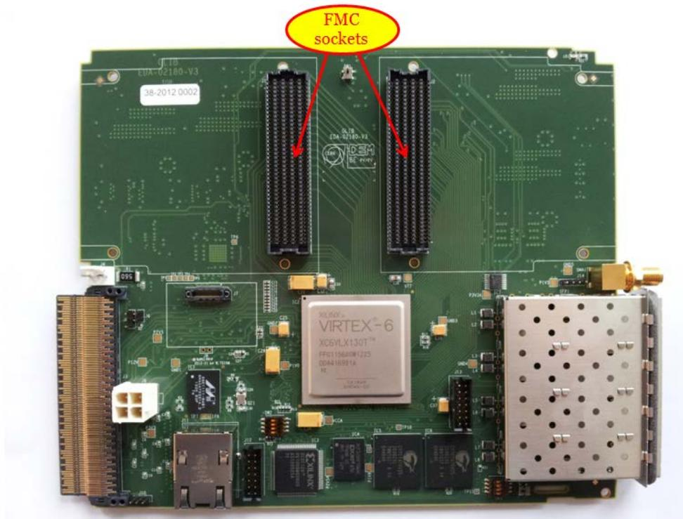
Figure 3: Picture of the GLIB AMC, highlighting the two FMC sockets
