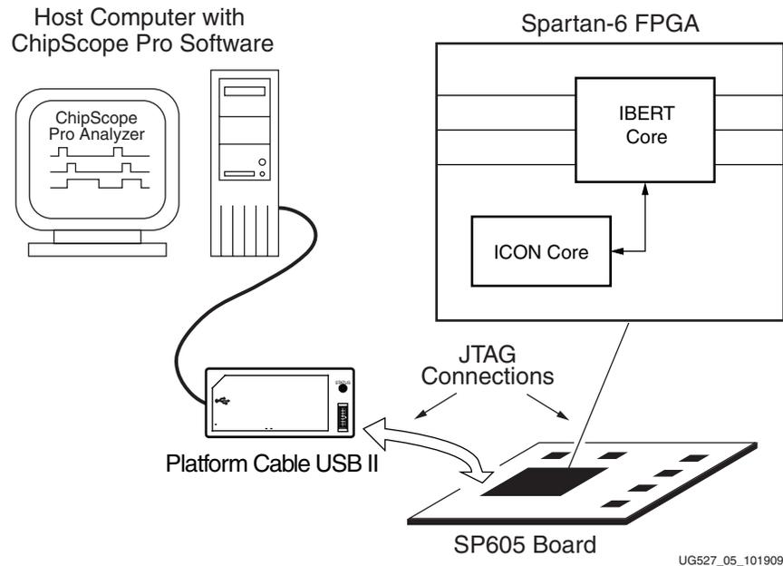
Figure 1-7: IBERT Core Generated Using ChipScope Pro Software
