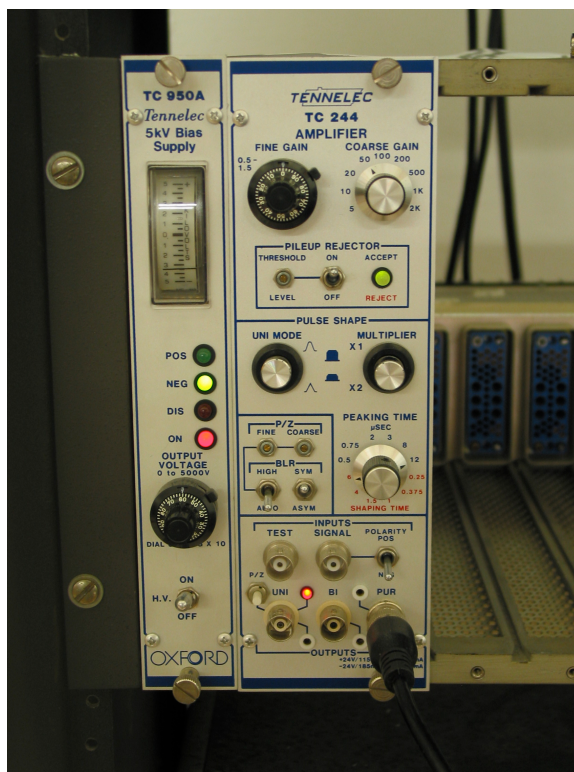
Figure 5 High Voltage Power Supply (TC 950A) and the Analog Shaping Amplifier (TC 244)
