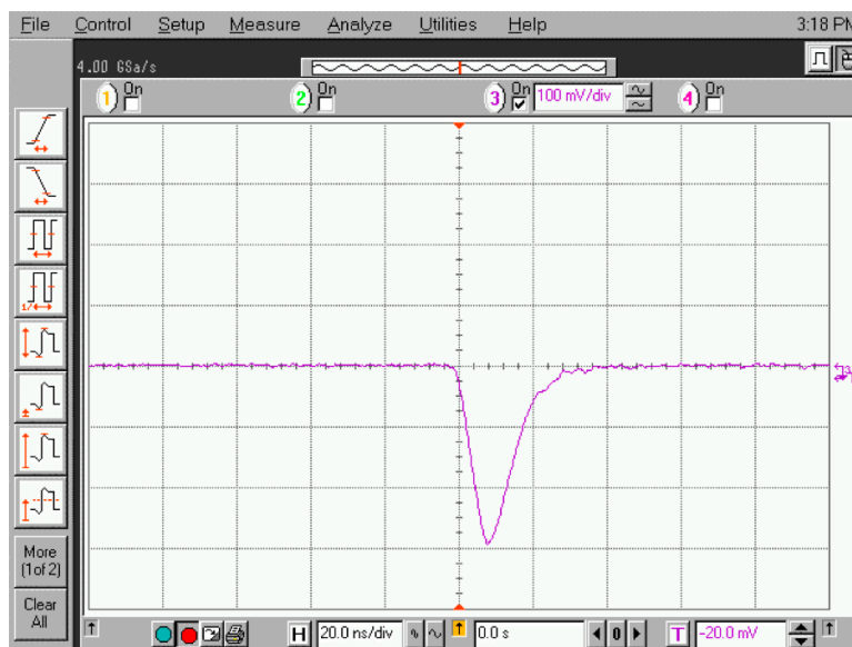
Figure 9 Output pulse directly from PMT into a 50\ \Omega load. Horizontal scale is 20 ns/div and vertical scale is 100 mV/div.
