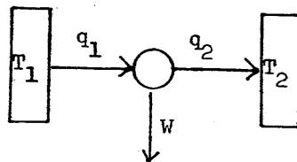
(a)  $W = q_1 - q_2 = C(T_1 - T_f) + C(T_2 - T_f) = C(T_1 + T_2 - 2T_f)$  (1)
