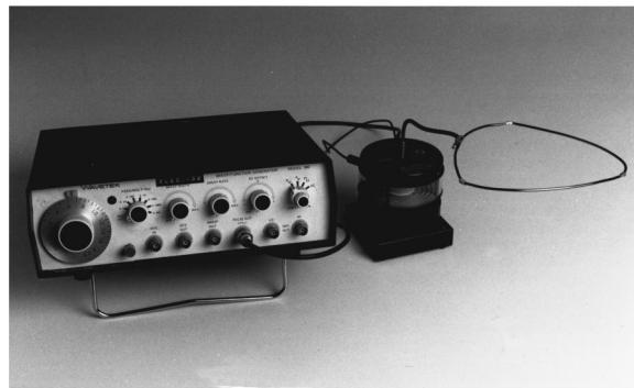
Fig. 5. Experimental setup used to show the quantum features of chaos. Notice that the membrane is excited in a way that breaks the symmetry.
