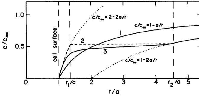
FIGURE 2 Relative concentration in the vicinity of a spherical absorber, for three cases: (1) No stirring; the current absorbed is  $J_0 = 4\pi a D c_\infty$ . (2) Volume between  $r_1$  and  $r_2$  stirred infinitely rapidly, fluid stationary elsewhere; current absorbed is  $2J_0$ . (3) Finite stirring speed; region inside  $r_1$  still dominated by diffusion; current absorbed is  $2J_0$ .
