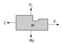
We are using kinetic friction as the system is moving, and it is directed to the left as the system is moving to the right. Let's call the sum of all the masses M = 10kg.
