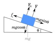
Here we choose the force to come out of the slope rather than down into it. Intuitively, if you press an object against a surface, it'll tend to stick more (you can even keep an object from falling down by pressing it against a vertical wall), so that seems to be the wrong direction to push it.
