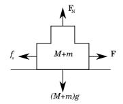
Our force must balance with  $f_{s,\max}$  in order to start the system moving. Newton's 2nd law in the horizontal yields:  $F - f_{s,\max} = 0$ In the vertical:  $F_N - (M + m)g = 0$ Altogether:
