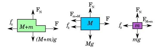
Now let's calculate the acceleration using the FBD of the entire system and Newton's 2nd law:
