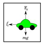
Of course, in the vertical direction, we have the force due to gravity mg pulling the car down and the normal force  $F_N$  which the road pushes onto the car. In the horizontal direction we have the force due to kinetic friction,  $f_k$ , which is what is slowing the car down. We can then write Newton's Second Law in the horizontal direction to figure out the leading car's acceleration (taking right to be positive):
