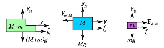
Like above, we will apply Newton's 2nd law to the entire system in order to find the acceleration of the blocks:
