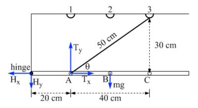
force at the hinge, which is shown broken into components on the diagram. To eliminate these unknowns sum torques about an axis through the hinge. Take counter-clockwise to be positive (you could set clockwise to be positive if you want).
