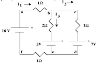
a. [2 pts] Write down the junction rule for the currents as marked
