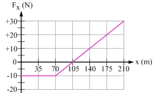
Figure 6.12: A graph of the net force acting on Peter and his bicycle, as a function of position.
