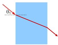
[2 points] (b) Briefly justify your answer: The ray bends towards the normal at the first interface, and then exits the block along the parallel sides. Snell's law is applied exactly the same way at both interfaces, so the angle at which the ray emerges from the block is  $\theta_1$ . Thus, the ray follows a path parallel to the original path, but displaces from the original path because of the change in direction inside the block.
