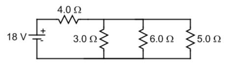
passes through the 4  $\Omega$  resistor. Method 2 – put the 5  $\Omega$  resistor in parallel with the 4  $\Omega$  resistor, increasing the current to the 3  $\Omega$  and 6  $\Omega$  resistors. Method 3 - put the 5  $\Omega$  resistor in series with the 3  $\Omega$  resistor, increasing the current to the 6  $\Omega$  resistor. Method 4 - put the 5  $\Omega$  resistor in series with the 6  $\Omega$  resistor, increasing the current to the 3  $\Omega$  resistor.
