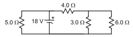
18 V across it and is unaffected. The overall resistance of the circuit goes down, and the current from the battery goes up, but all the extra current goes through the 5  $\Omega$  resistor.
