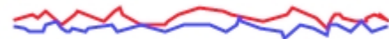
Figure 5.4: A magnified view of two surfaces in contact. The irregularities in the objects prevent smooth motion of one surface over the other, giving rise to friction.
