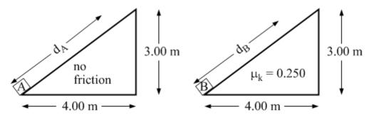
Two identical blocks, A and B, are placed at the bottom of almost-identical ramps and given **initial velocities of 6.00 m/s up their ramps**. Both ramps are in the shape of 3-4-5 triangles, as shown, but block A's ramp is frictionless while the coefficient of kinetic friction between block B and its ramp is 0.250. Both blocks slide up and down their ramps. Use  $g = 10.0 \text{ m/s}^2$ .
