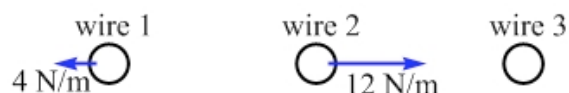
Figure 19.42: Three long straight wires carry currents perpendicular to the page. The net forces per unit length on two of the wires are shown. For Exercise 20.
