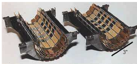
(a) A photograph of the SVT showing the array of silicon chips.
