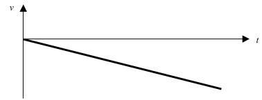
3. Yes, in this case one can analyze Smoky's up and down motion without breaking it up into an upward part and then a downward part. The reason is that his acceleration is the same (and constant) for that entire motion. As long as acceleration remains constant, the equations for motion with constant acceleration can be used continuously.
