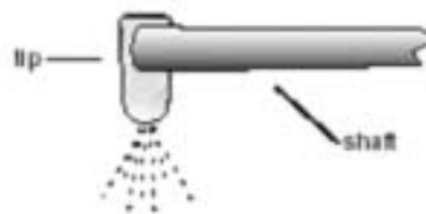
Figure 9. Correct position of the atomizer tip
