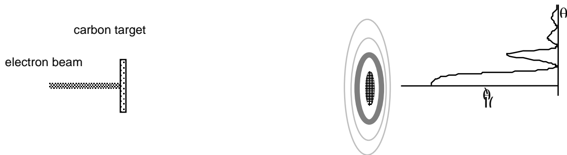
Figure 3. Wave Model Diffraction. Constructive interference of an electron beam through a polycrystal.
