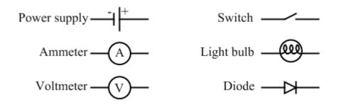
A current at any point in a circuit can be measured with an ammeter. Ammeters are placed in series with the device through which the current is being measured, to ensure that the current through the ammeter is the same as the current through the device. The ammeter should also have a very small resistance, so it will change the current in the circuit by a negligible amount.
