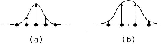
FIG. 2. Shapes of low-frequency localized modes in a nonlinear chain when (a) centered on a site and (b) centered between sites. Note that in each case the mode shows the in-phase oscillation of neighboring sites that is associated with an acousticlike excitation, as one would expect for a low-frequency mode. For these modes, case (a) has lower energy than case (b).
