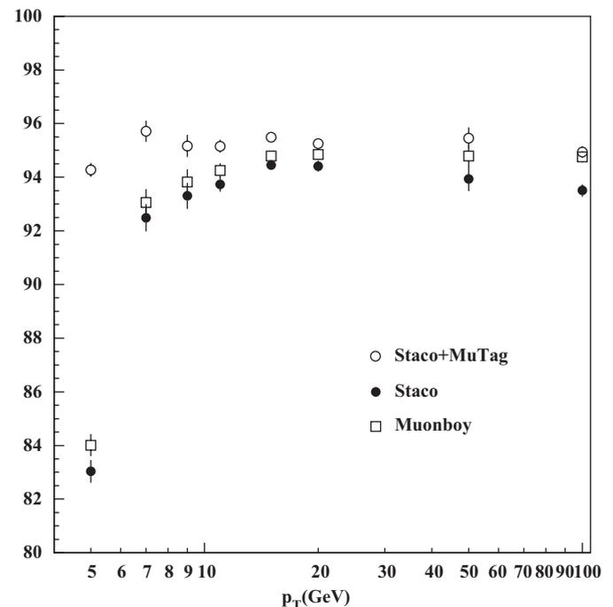
Fig. 3. Efficiency of track reconstruction using MUONBOY, STACO and MuTag as a function of  $p_T$ .
