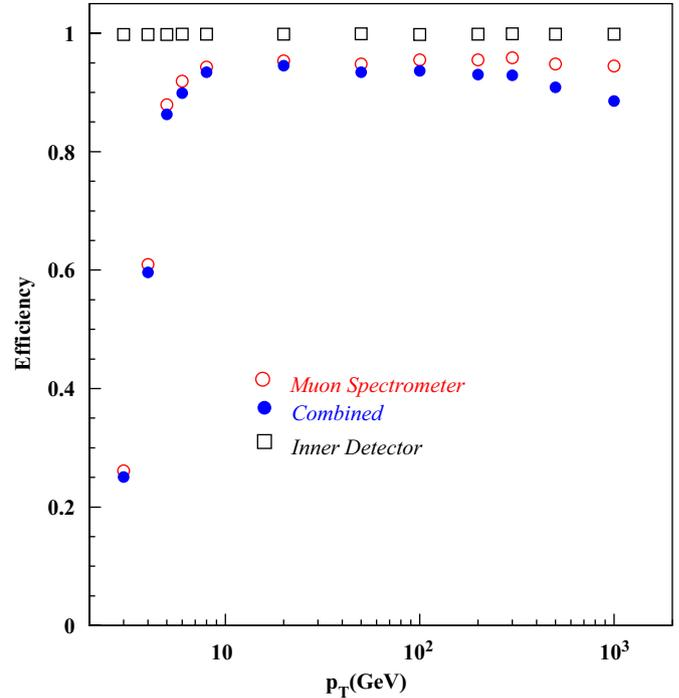
Fig. 2. Efficiency of track reconstruction in the Muon System and in the Inner Detector, using the STACO procedure, as a function of  $p_T$ .
