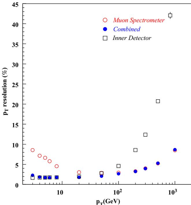
Fig. 1.  $p_T$  resolution of track reconstruction in the Muon System and in the Inner Detector, using the STACO procedure, as a function of  $p_T$ .
