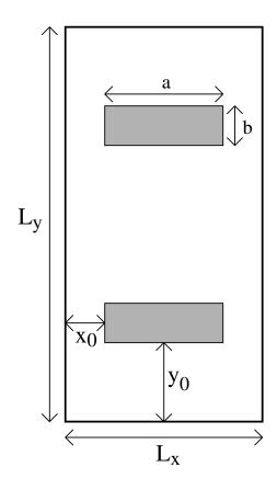
Figure 1: Geometry of the semiconductur nano-structure. The potential  $V = -V_0$  in the shaded areas an V = 0 elsewhere inside the quantum dot. The two low-potential areas are identical and symmetrically located as shown. Outside the boundaries of the  $L_x \times L_y$  structure the potential is assumed to be infinite.
