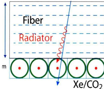
Transition radiation is emitted in the radiator and is subsequently absorbed in the proportional tubes, along with standard  $dE/dX$  radiation from the primary particle.
