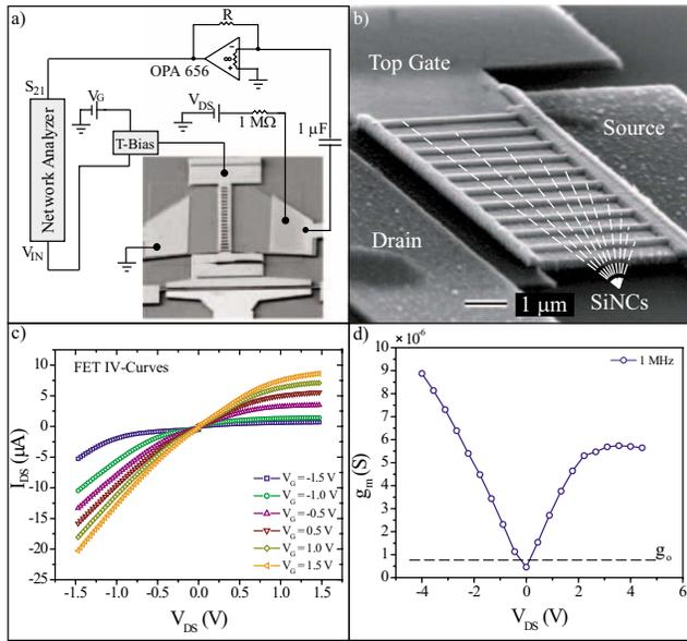
FIG. 3. (Color online) (a) Schematic of the SiNC FET characterization circuit. (b) 3D image of a SiNC FET. (c) Typical asymmetric  $IV$ -curves of the SiNCs. (d) Transconductance  $g_m$  of the SiNC FET for 1 MHz top gate voltage signals ( $V_{in}$ ) as a function of source-drain voltage ( $V_G=0.5$  V). The dotted line represents the minimum (unity gain) transconductance  $g_o$  required to use the SiNC FET as an amplifier at 1 MHz.
