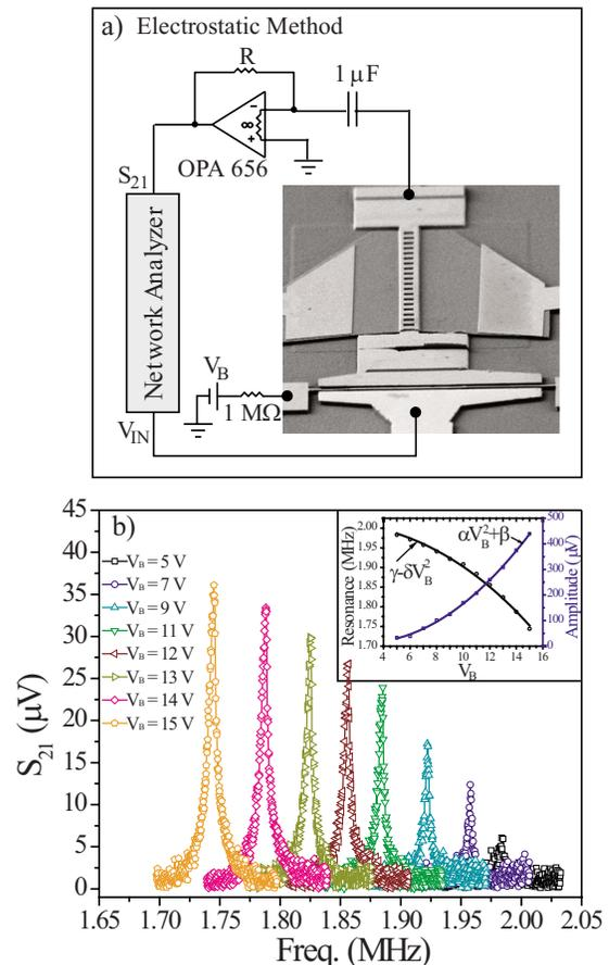
FIG. 2. (Color online) (a) Schematic of the electrostatic measurement circuit. (b) Typical response of the beam measured via the electrostatic method. Inset: Dependencies of resonance amplitude and frequency on  $V_B$ , with corresponding fits.
