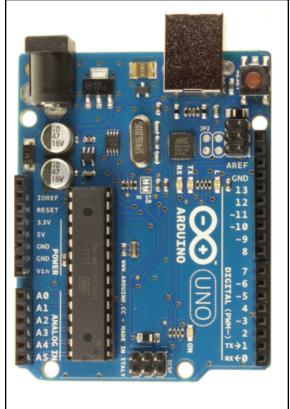
This is an Arduino. Note the labeled sockets which can easily be connected to your breadboard with wires.
