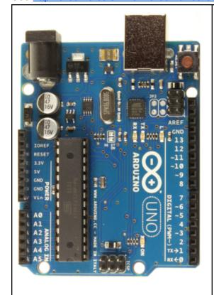
This is an Arduino. Note the labeled sockets which can easily be connected to your breadboard with wires.
