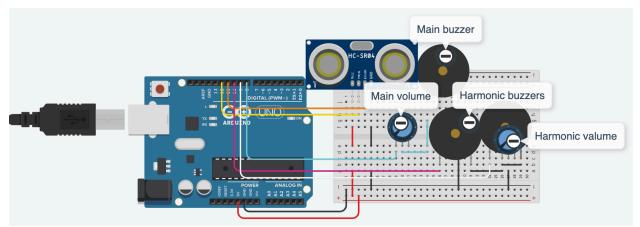
In actual implementation the ultrasonic distance sensor will be placed at a more convenient location for measuring distance with comfortable hand position. The code on implementing the basic Theremin setup would primarily evolve converting distance measured to reasonable frequency and deal with cutting off unattainable distance measurements.
