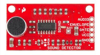
The envelope pin transmits an analog signal depending on the amplitude(loudness) of the sound.
