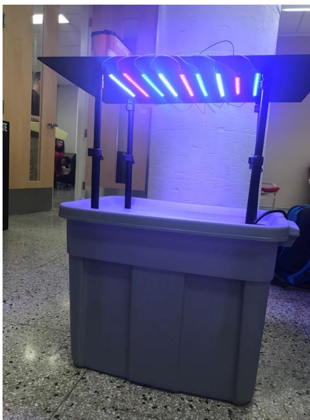
Figure 2: Photo of my final project. LED's on top are PWM controlled and the plastic tub houses a submersible pump that sprays nutrient rich water on the roots of the plant.
