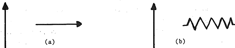
Fig. 1. The bond elements of (a) fully and (b) partially directed percolation on the square lattice. The arrow corresponds to a diode, the zig-zag to a resistor.
