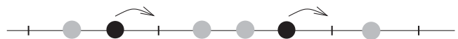
FIG. 1. Illustration of occupancy facilitated asymmetric exclusion. Particles that are eligible to hop to the right are dark, while immobile particles are shaded. This configuration contains islands of lengths 2, 3, and 1 (left to right).
