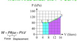
The net work done by the gas is positive in this case, because the change in volume is positive, and equal to the area under the curve.
